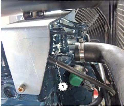
Figure 27: Flexibles gasoil
